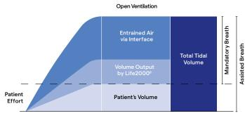
Assisted Breath (V<sub>T</sub>)=Patient's Volume +Volume Output + Entrained Air Mandatory Breath (V<sub>T</sub>)=Volume Output + Entrained Air
